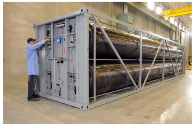
**FIGURE 3.** Final Assembly of TITAN ISO Frame System
